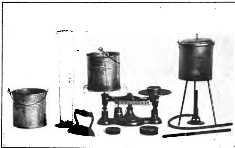
FIG. 19. Apparatus used to illustrate the heat units, and to show that different substances at the same temperature may contain different quantities of heat.
